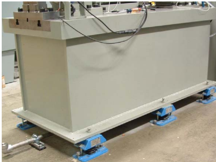
Figure 9 Test base supported on vibration isolators to reduce base natural frequency and orthotropy
