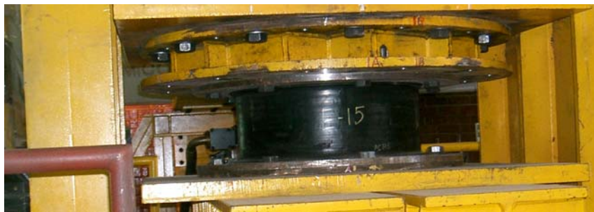
Fig. 10. HDRB subject to shear loading
