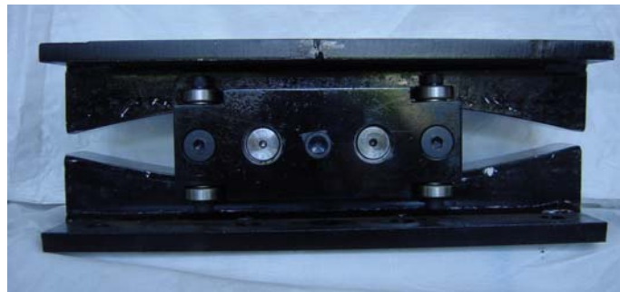
Fig. 9. FPS bearing with dual rollers
