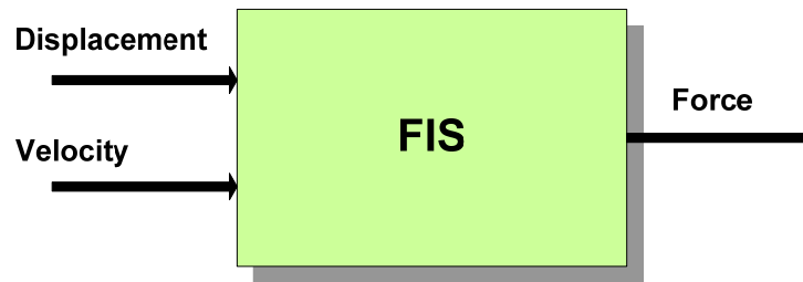
Fig. 15. Example inputs and output for a FIS of an isolation device
