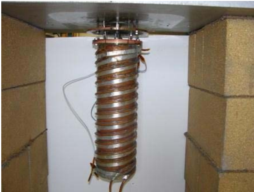
FIGURE 24. Heating/Cooling shield -2 with heating tape 1 and 2 connections made.
