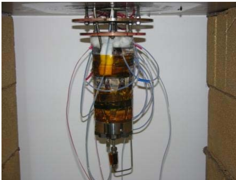
FIGURE 25. High pressure MDS cell with PRT and thermopile connections made.
