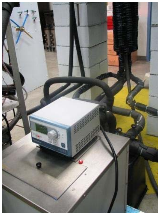
FIGURE 26. PolyScience ® constant temperature bath and its connections to MSD.
