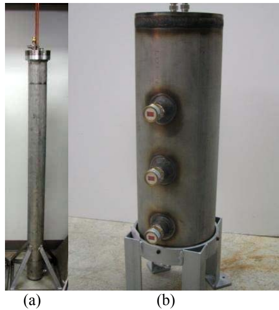
FIGURE 30. Liquid nitrogen/ liquid propane heat exchanger (a), liquid propane tank (b).
