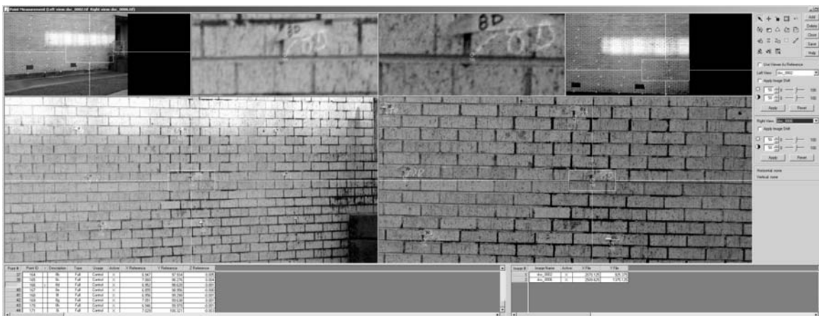
Fig. 8.—Triangulation accuracy test photographs. The two photographs used for the triangulation accuracy test. Note the high angle between photos.
