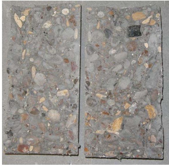
Figure 5.4 Fracture surface of concrete with VG
