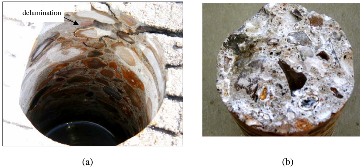
Figure 6.7 The coring sample with delamination: (a) top view of the coring hole; (b) fracture surface
