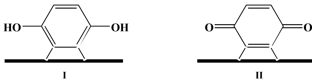
Fig. 22. Models for the ortho-di- \sigma -bonded species in the reduced (I) and oxidized (II) forms. The bottom black line represents the Pd surface.
