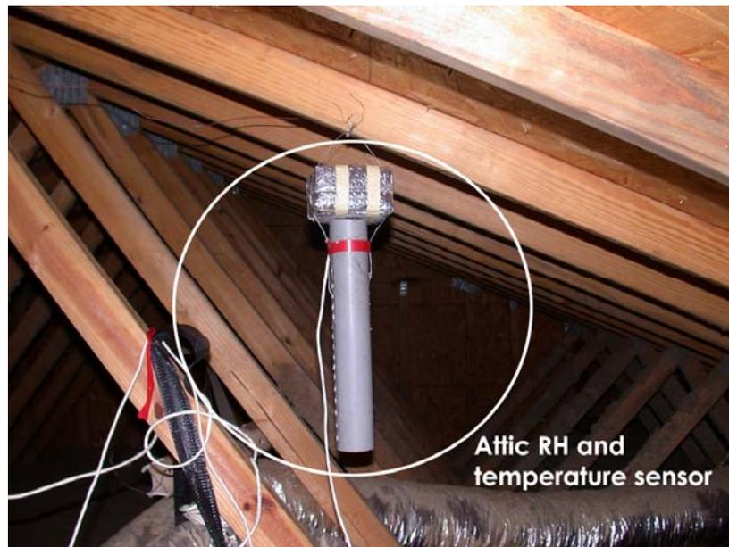
*Figure 4.10 Attic temperature / relative humidity sensor with radiation shield and insulation*
