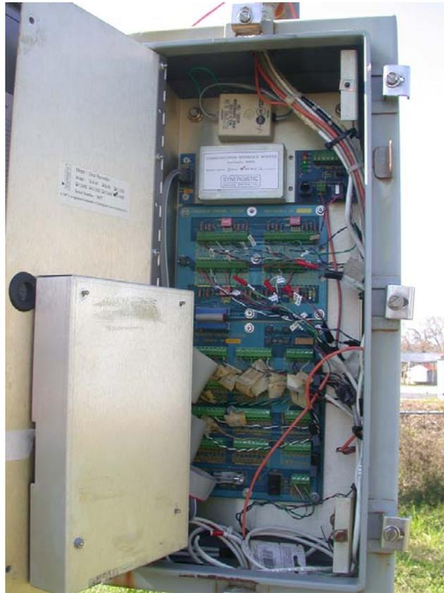
**Figure 4.8** Data logger (Synergistics Data Logger C180E)
