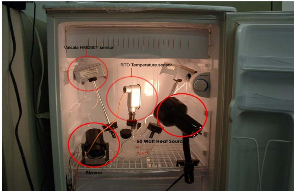
**Figure A.2** Experimental setting showing the Vaisala and RTD sensors
