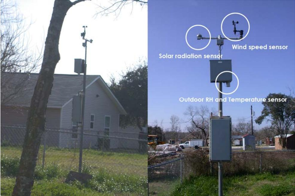
Figure 4.7 Data logger (Synergistics C180E) with weather station on case-study house
