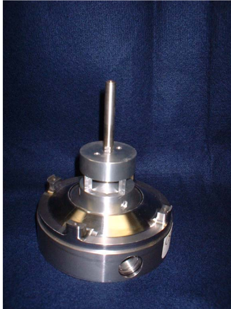
Figure 16: Demonstration of ability of second stage to be nested within the first stage.
