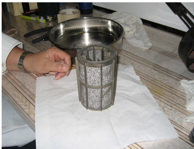
Figure 4.3 Stainless steel Catalyst Basket modified by the Chemical Engineering workshop at A&M University.
