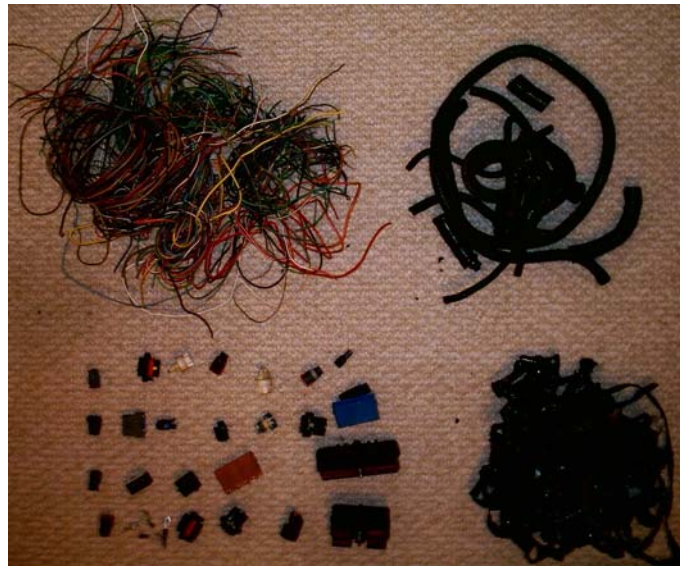
Fig. 9. Fully disassembled engine wiring harness from a 1995 Dodge Neon. Shown clockwise from top-left: wires, casing, tape, and connectors.
