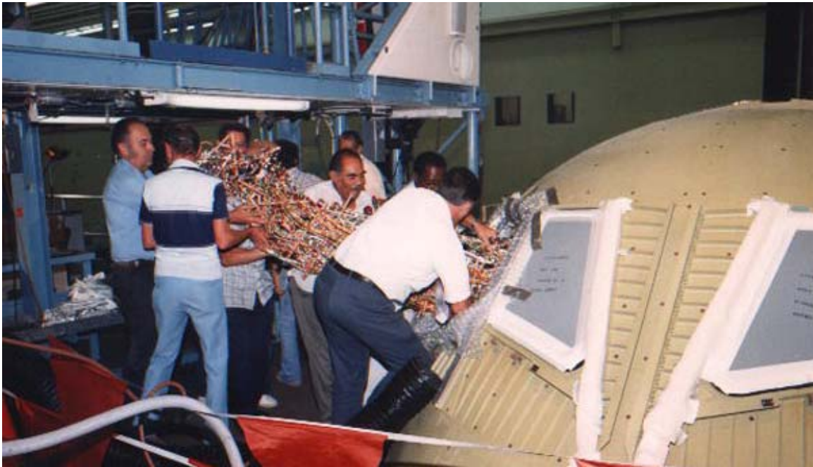
Fig. 4. Installing a wiring harness for the Endeavour space shuttle [6].
