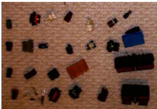
Fig. 3. Connectors from an engine compartment wiring harness in a 1995 Dodge Neon.
