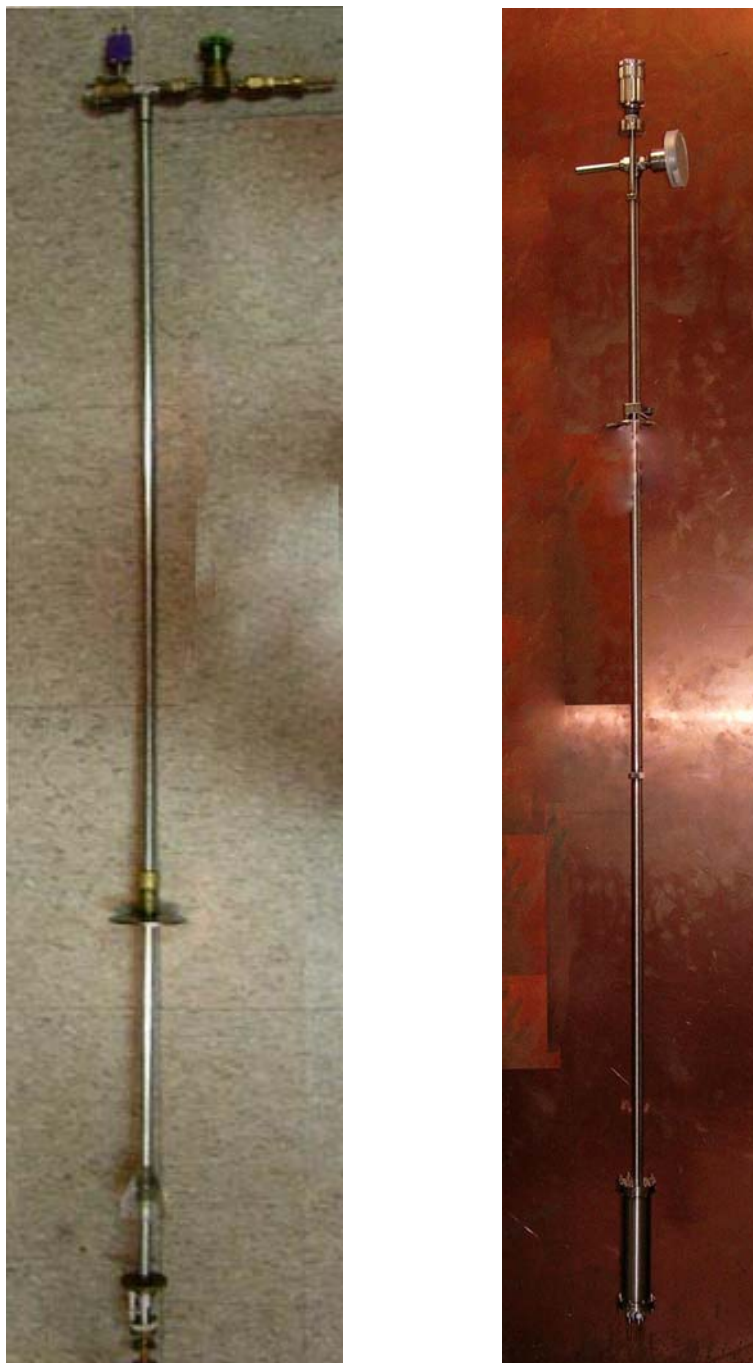
Figure 3.1 Exterior view of an insertable cryostat (left) and our quench-condensation apparatus (right)
