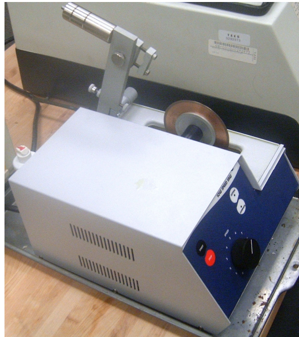
Figure IV.12 - Buehler Isomet low speed saw
