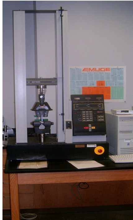
Figure IV.15 - Instron Universal testing machine M10-24411
