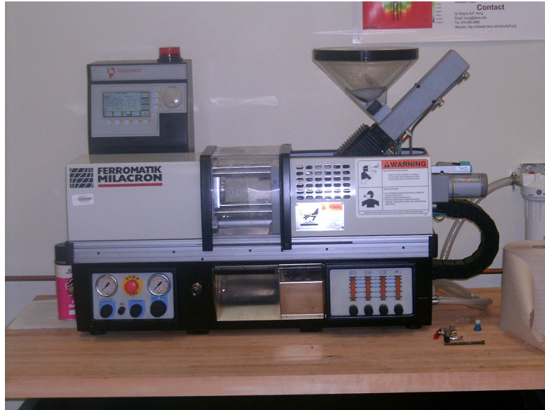
Figure IV.9 - Injection molding machine manufactured by Ferromatik Milacron, Model Babyplast
