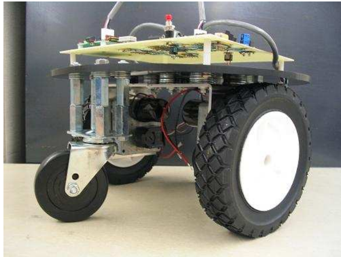
Fig. 26. Mobile robot base: Rex-12 from Zagros Robotics
