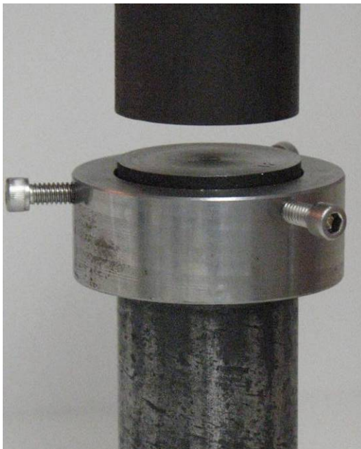
(c) Pestle and Mortar Interface
