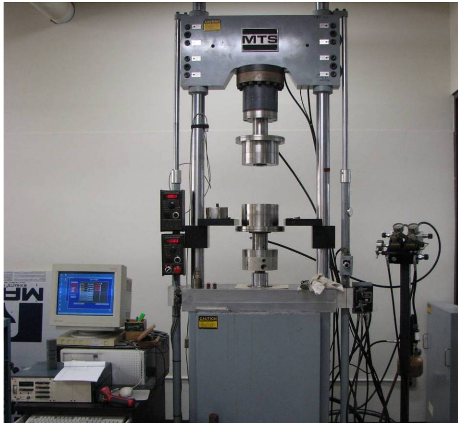
Figure 3.6: Axial-Torsional Load Frame and Data Acquisition
