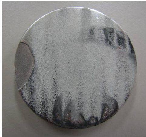
Figure 4.4: Specimen #7 Damaged Prior to Testing
