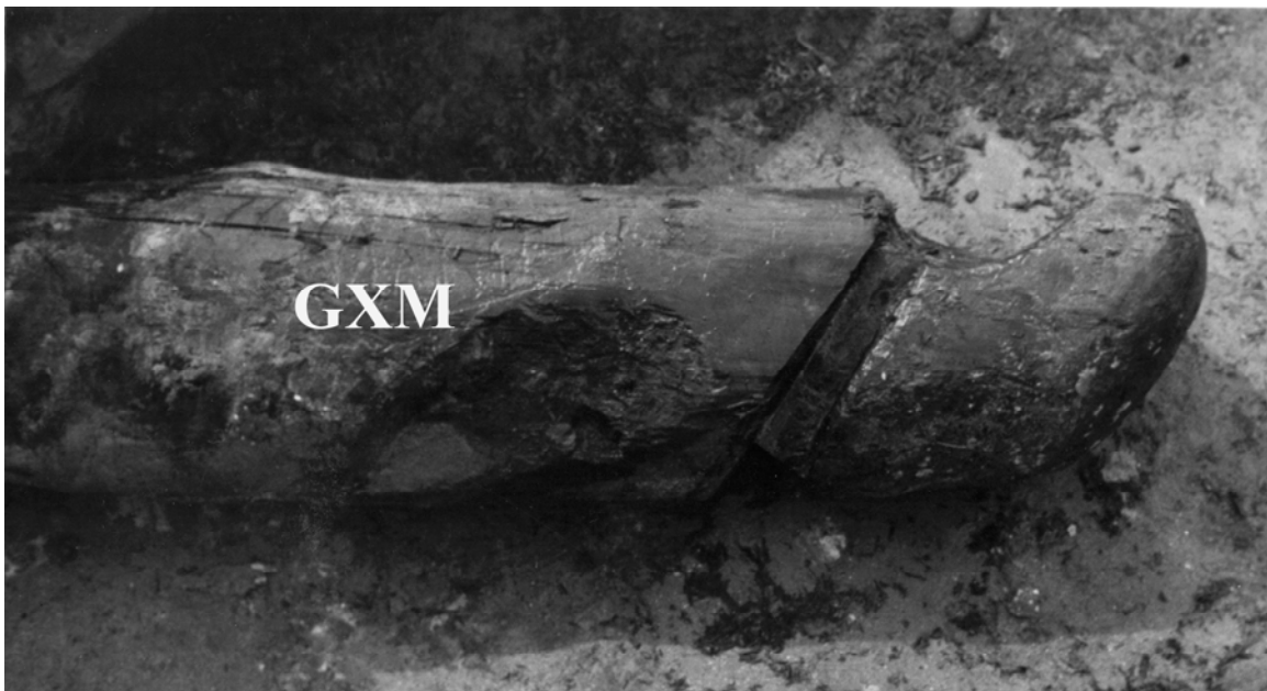
Fig. 6.7 The Pantano Longarini ship's through-beam GXM shaped to fit in the planking and wales (after Throckmorton and Throckmorton 1973, Fig. 22).
