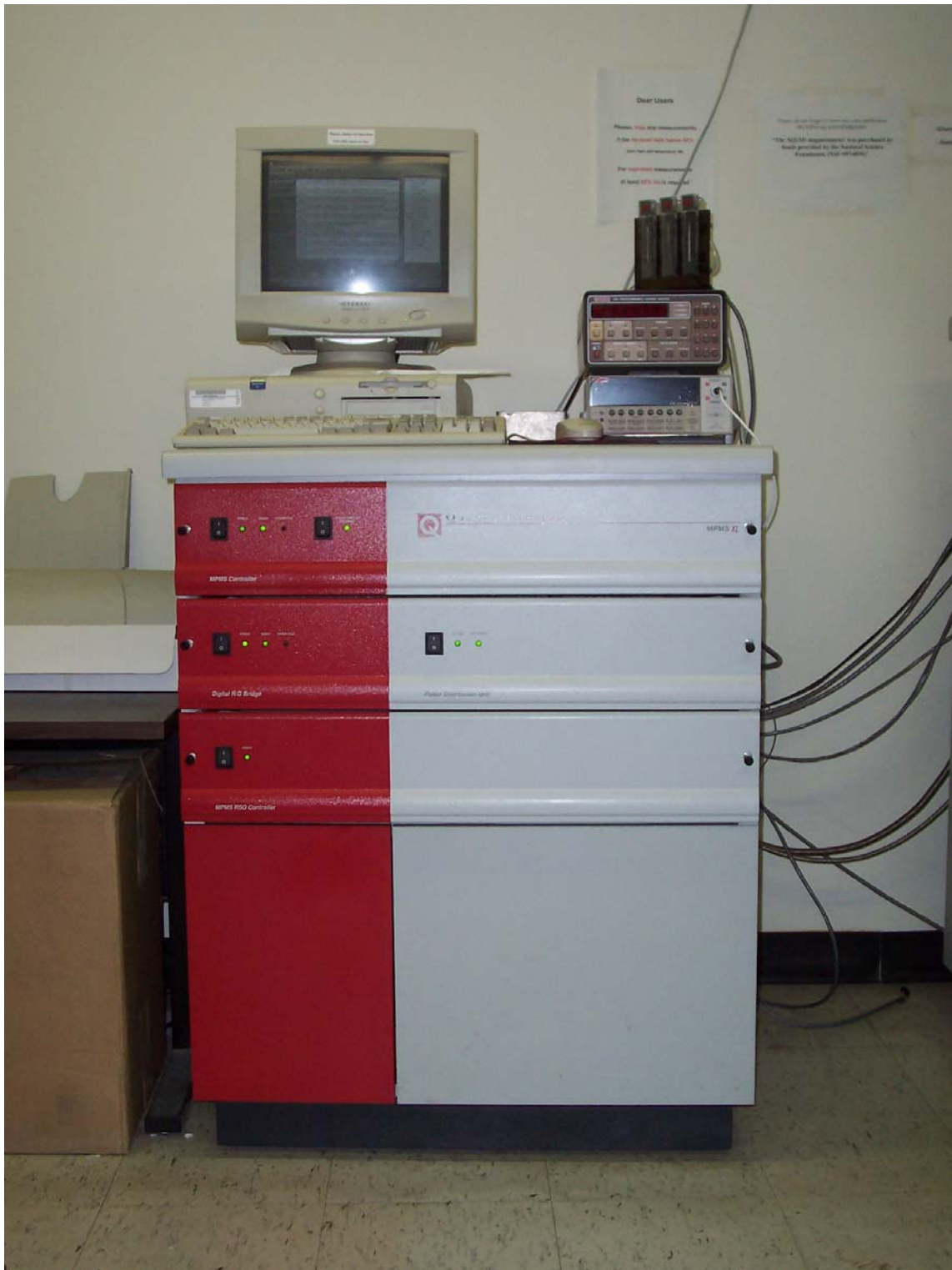
Fig. 97: SQUID magnetometer, processing electronics
