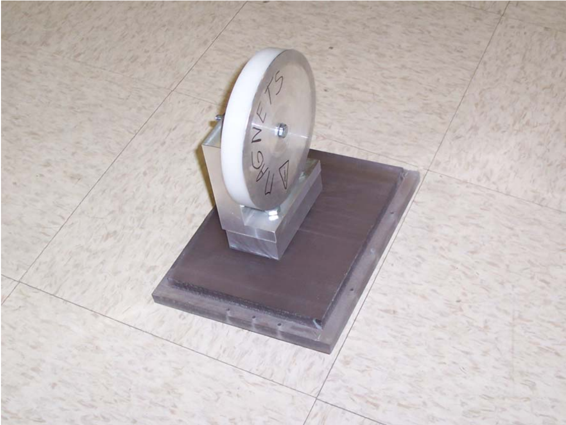
Fig. 93: Complete stator assembly and mount
