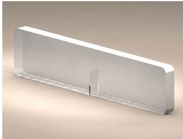
Figure 7 SENB specimen showing a sharp natural crack.
