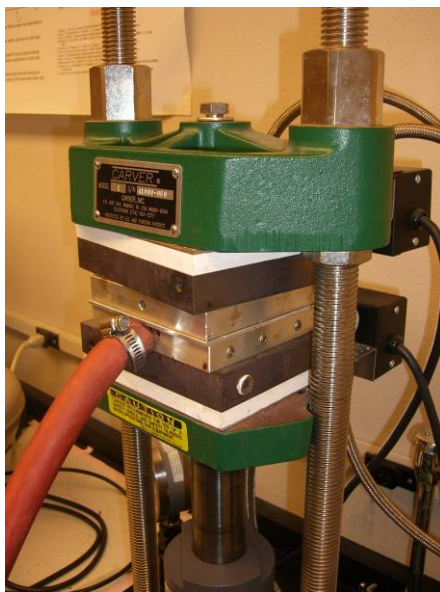
Figure 3 Compression molding in a hot press with a vacuum applied to the mold.
