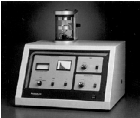
Fig. 17 Hummer sputtering system
