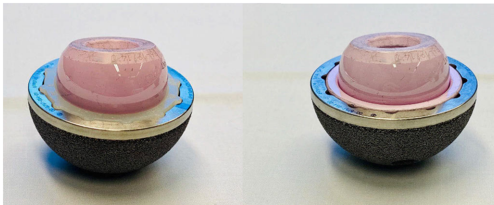
Figure 11. Ceramic-on-polyethylene (left) and ceramic-on-ceramic (right) bearings with Continuum cup.
