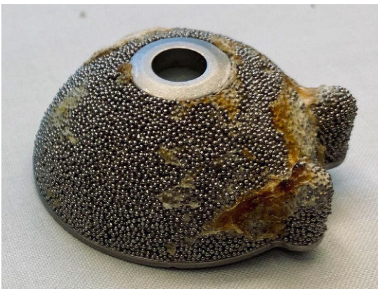
Figure 7. The porous-coated anatomic (PCA) cup component was one of the first uncemented acetabular components. The cup was fabricated from cobalt-chromium alloy and featured a sintered-bead porous surface to allow bone ingrowth. Superiorly placed fixation lugs enhanced primary stability.
