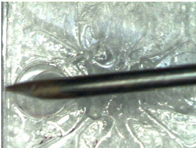
Fig. 44. Image showing the introduction of a drop of HEPES solution with the help of a micro-syringe into one of the chambers.
