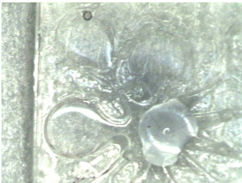
Fig. 54. Image showing the HEPES solution and peptide inside the reaction chamber of the microfluidic device.
