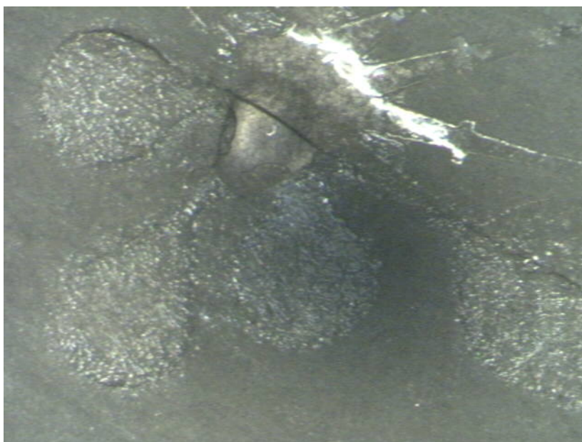
Fig. 76. Image showing the flow of the HEPES solution into the reaction chamber by capillary action.
