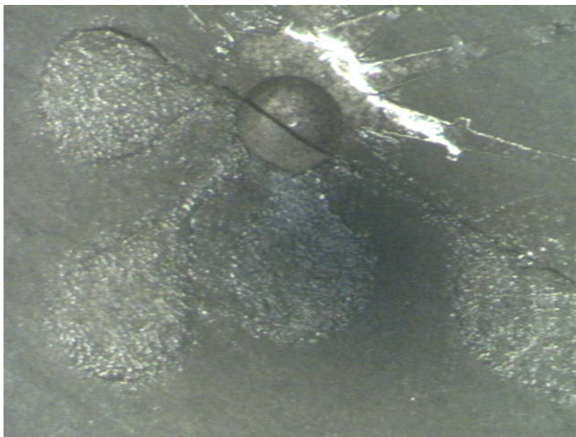
Fig. 77. Image showing the droplet inside the reaction chamber of the microfluidic substrate.
