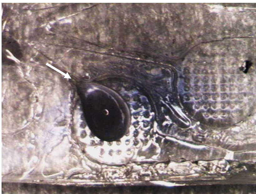
Fig. 40. The darkish liquid (gold precipitate) flows out of the reaction chamber into the drainage chambers.
