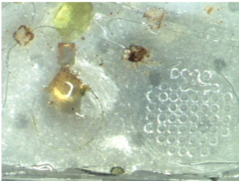
Fig. 72. Image showing the drop of gold acid inside the reaction chamber. The valve has dissolved out completely.
