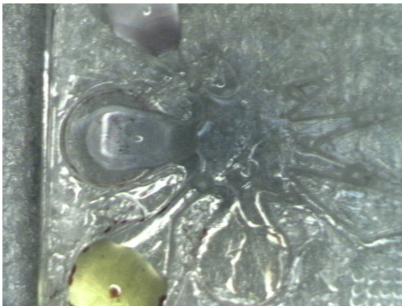
Fig. 51. Image showing the HEPES solution entering the reaction chamber.
