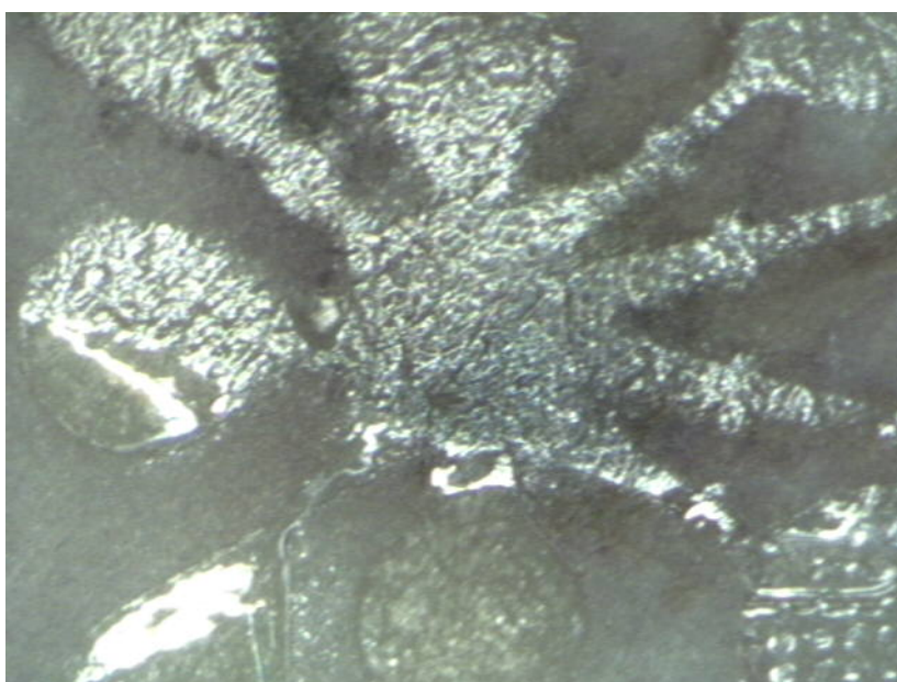
Fig. 91. Image showing a magnified view of the reaction chamber on the paper microfluidic substrate.
