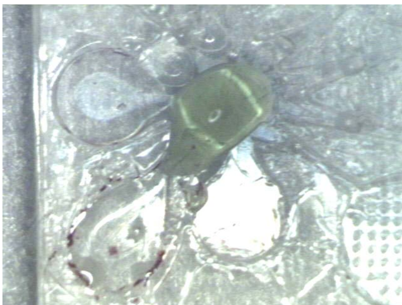
Fig. 55. Image showing the rupture of the valve allowing the Chloroauric acid to flow into the reaction chamber.
