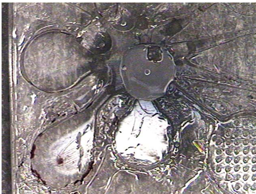
Fig. 36. HEPES fills the reaction chamber of the microfluidic substrate. The surface is made hydrophilic by oxygen plasma treatment prior to the experiment.
