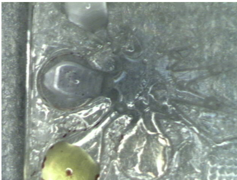
Fig. 50. Image showing the HEPES solution gradually dissolving the valve and flowing into the reaction chamber.
