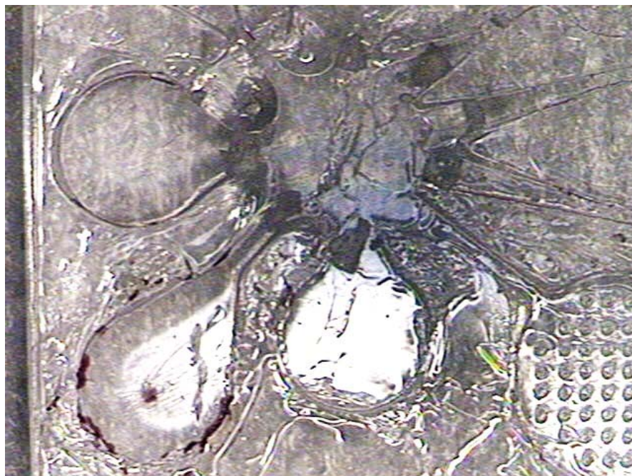
Fig. 32. Image showing the reaction chamber of the microfluidic device. Each of the reservoirs is connected to this central chamber by micro-channels with passive actuation valves placed inside them.
