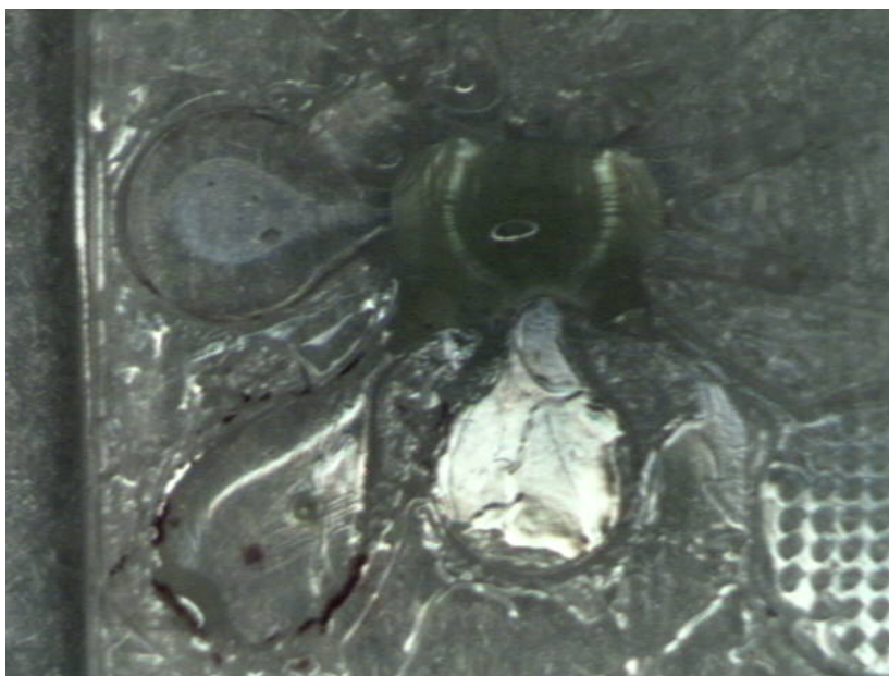
Fig. 57. Image showing the darkish precipitate moving into the drainage chambers.
