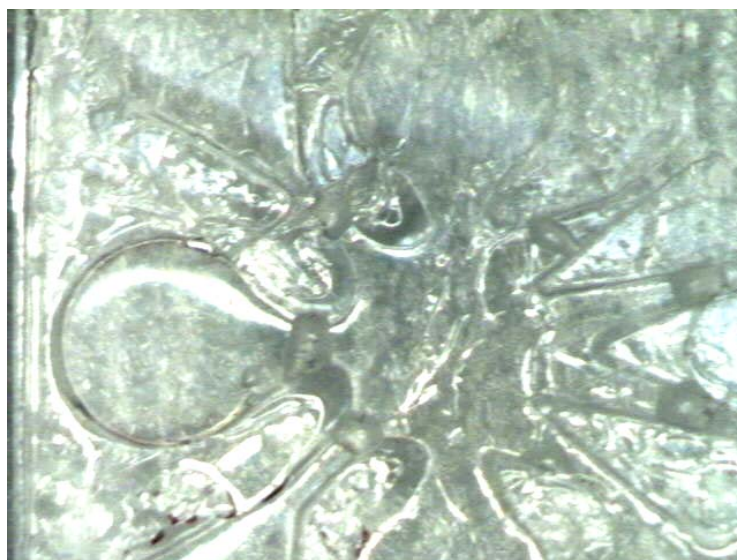
Fig. 43. Image showing a magnified view of the reaction chamber in the microfluidic substrate.
