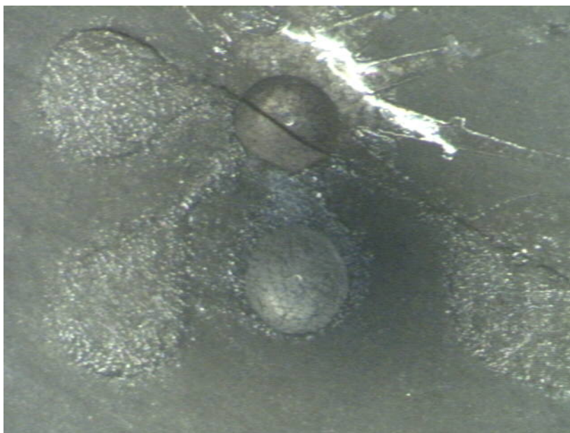
Fig. 78. Image showing the introduction of a droplet of poly-tyrosine inside another reservoir of the paper microfluidic substrate.
