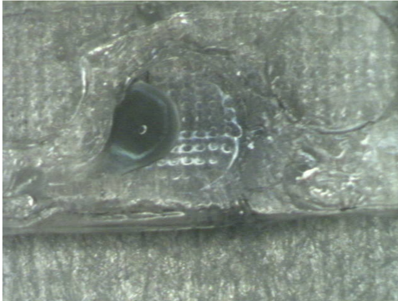
Fig. 64. Image showing a drop of liquid in the second set of drainage chambers in the microfluidic device.
