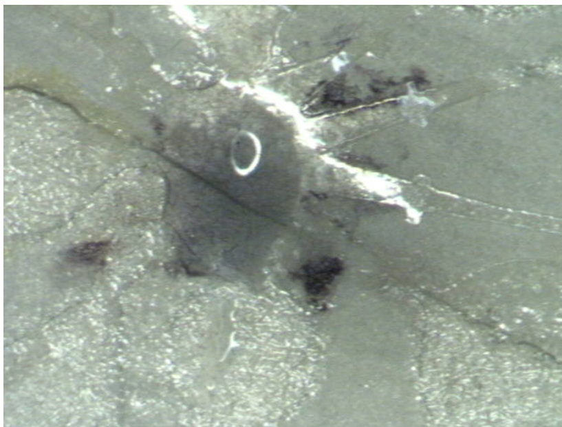
Fig. 90. Image showing the formation of gold nano-particles inside the reaction chamber of the microfluidic substrate on paper.
