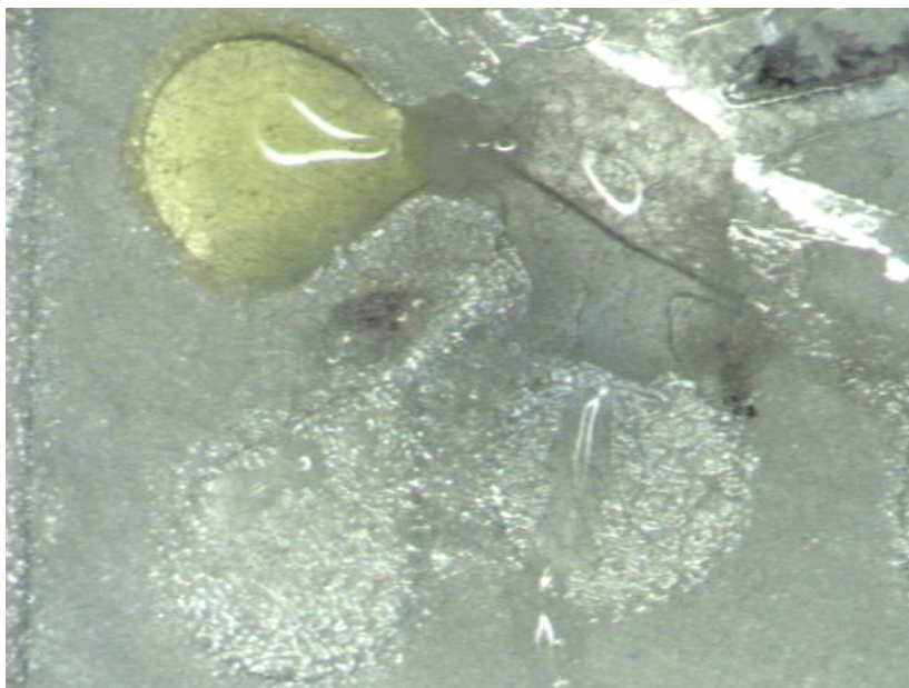
Fig. 89. Image showing the Chloro-auric acid droplet dissolving the salt bridge valve to enter into the reaction chamber.
