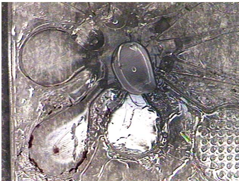
Fig. 35. The HEPES solution gradually flows into the reaction chamber and fills it up.
