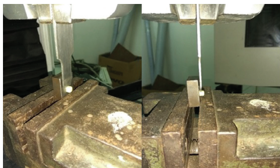
Fig. 4: Shear bond strength testing using Universal testing machine.
