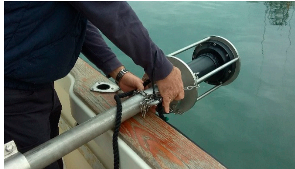
Figure 2. Tooling for joining the echosounder to the side of the boat.
