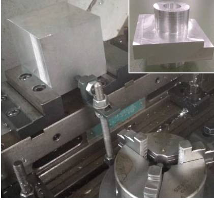
Fig. 12: Machining center, workholding devices and machined part from case study.
