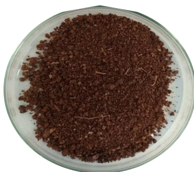
Figure 13 Dried pellet obtain from the centrifugation of grape pomace with deionized water.
