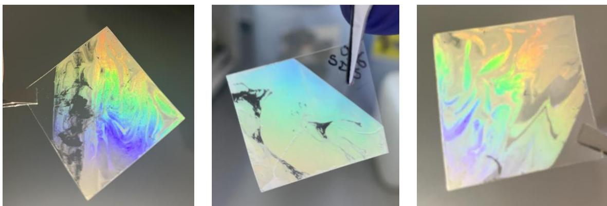
*Figure 3.3.7 – Resulting typical defected substrates after the previous Langmuir-Blodgett 0.6  $\mu\text{m}$  PS nanospheres depositions: the achieving of a direction-oriented colorful pattern (see Google Drive video 8) areas indicate the attaining of a high-ordered layer, whereas ACS is higher; on the other hand, the more transparent/whitish areas indicate a low-quality deposition, which should reveal disordered nanosphere clusters, therefore, low substrate area uniformity.*
