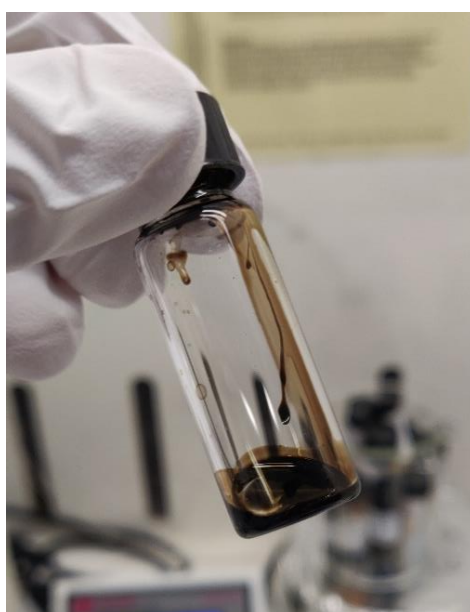
Figure C-4: Standard final solution before deposition (without mercaptopropionic acid).
