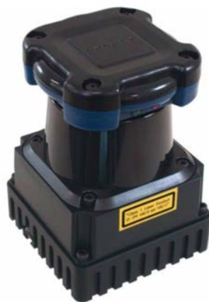
Figure 2.45: Hokuyo UTM 30LX-EW Laser Scanner. Courtesy of (Koch et al., 2017)
