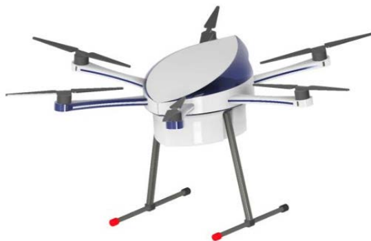
Figure B.4: Multi-Rotor UAV: HEIFU.
