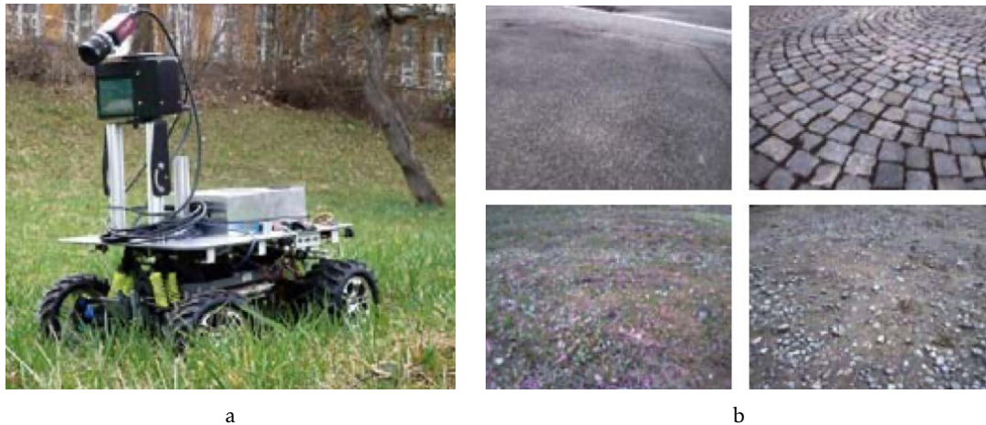
Figure 2.44: a) The USV used for ground image acquisition; b) The four terrain classes used in the ground dataset (Otte et al., 2015).
