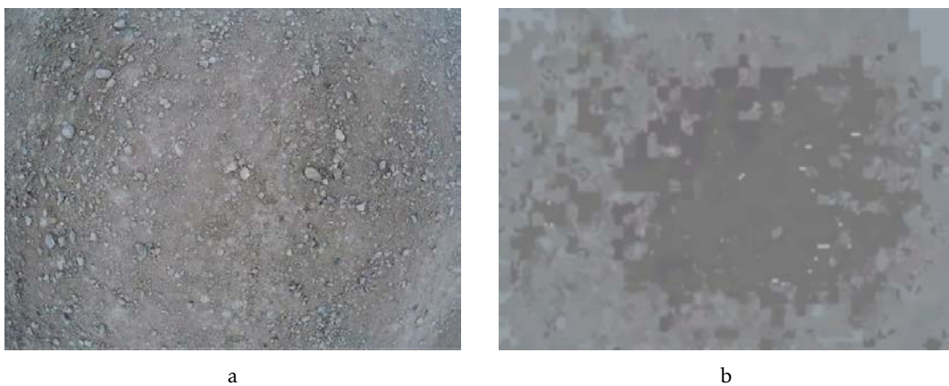
Figure 3.18: a) Input image (sand terrain A); b) PSO segmented data.
