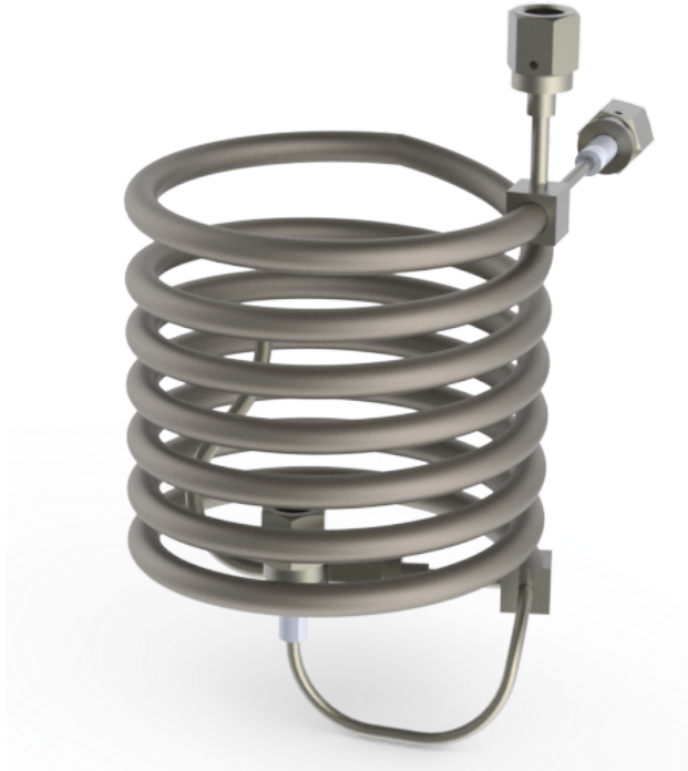
Figure 5.7: Rendered view of the 2 m tube-in-tube configuration heat exchanger designed for the JT stage at 80 K.
