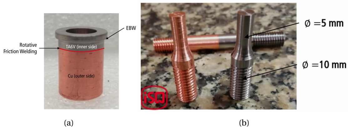
Figure 6.3: Cu/Ti bimetallic adapter: a) Machined bimetallic adapter; b) Tensile specimens machined for the tensile pull testing.
