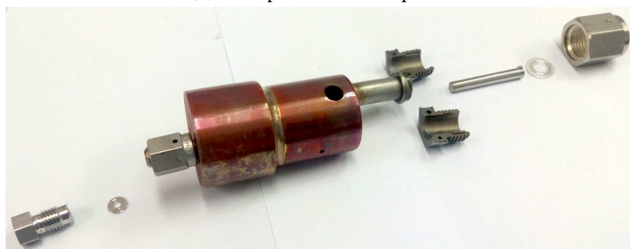
(b) Modular adsorption cell using Swagelok VCR® fittings.
