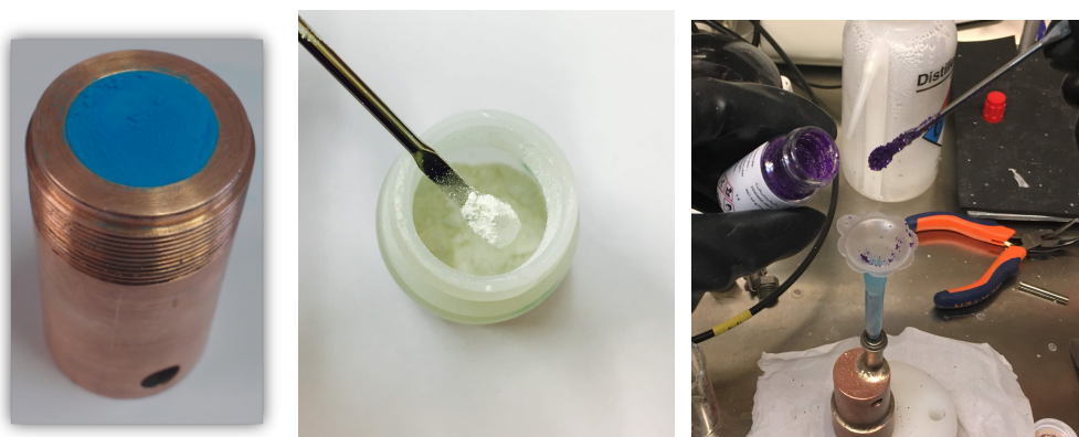
Figure 4.2: Left side: Purplish powder of HKUST-1; Middle: very fine white powder sample of UiO-66; Right side: Purplish powder of \text{Co}_3(\text{ndc})_3(\text{dabco}) on argon atmosphere glove-box.
