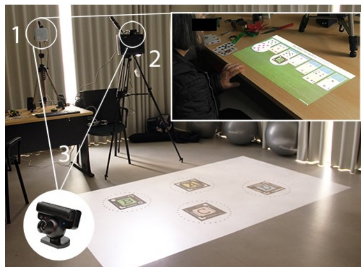
Figure 4.21. System configuration(s). (1) Table projection set up with a projector and a tripod. (2) Floor projection setup through a high-intensity projector and a tripod. (3) A PSEye camera is collocated with the projectors to track and identify the projected markers A, B, C, and D.
