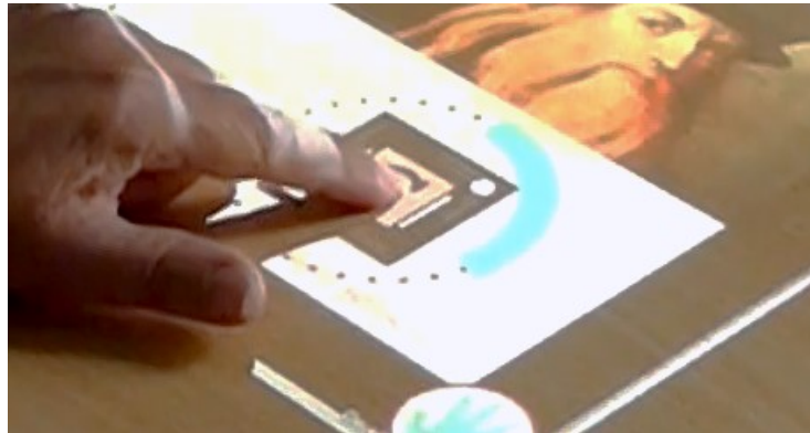
Figure 4.20. Circular timer and marker. A blue circular timer is activated after occluding the marker with the finger, full-body, or random physical objects.
