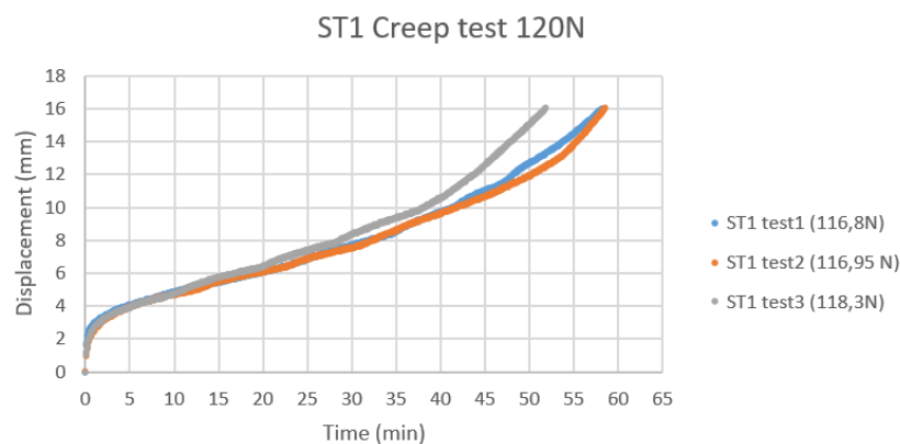
Figure 6.3: ST1 creep test curves for a load applied of 120 N
