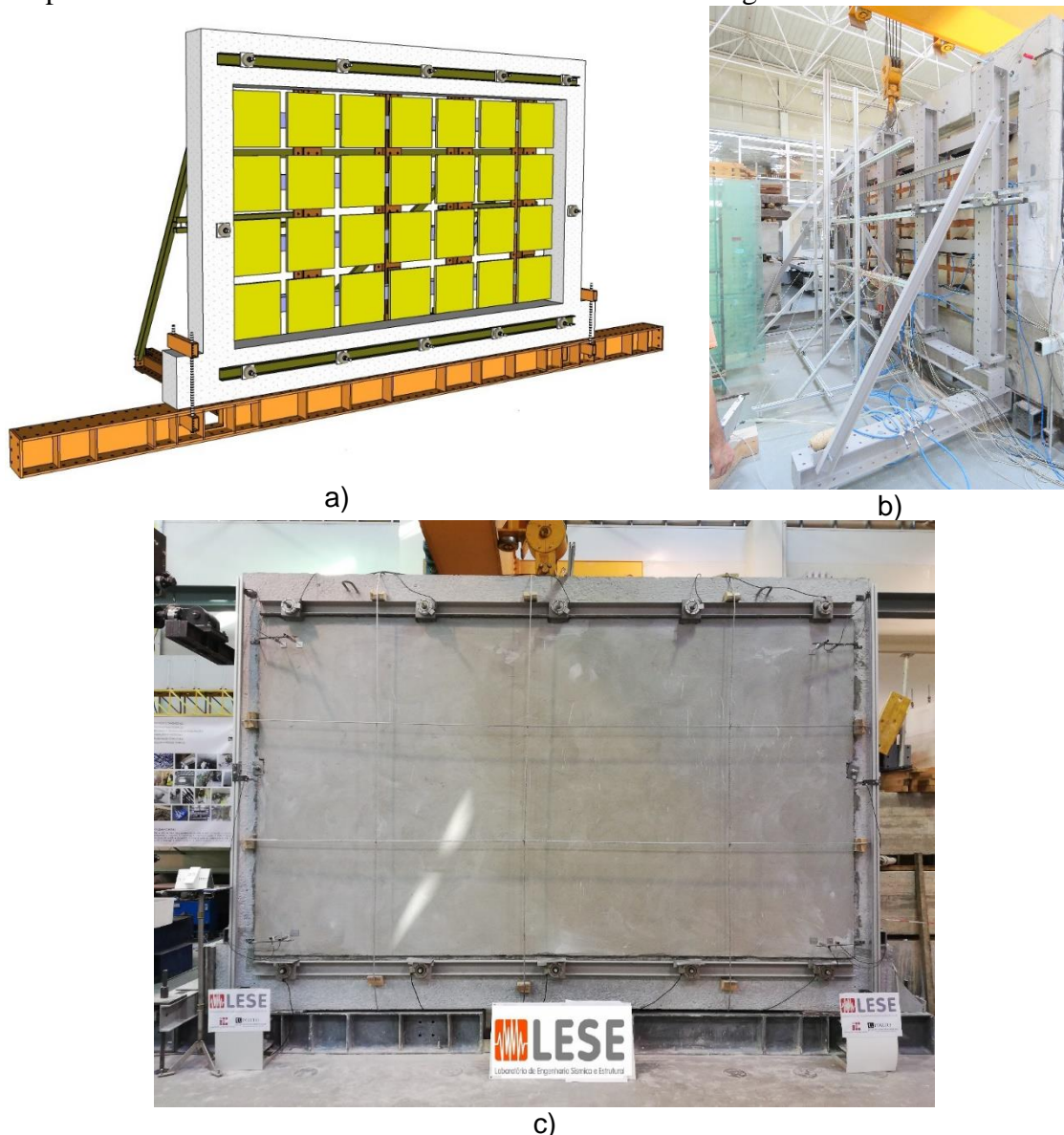
Figure 4: Test setup: a) schematic layout; b) lateral view; and c) front view.
