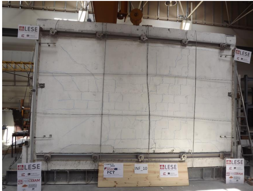
Figure 8: Specimen Inf_10: Cracking pattern.
