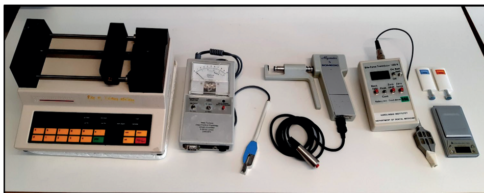
Figure shows a Harvard infusion pump, an Umeå bite force transducer for fine precision forces, a Somedic electronic pressure algometer, an Aalborg bite force transducer for MVBF, a mechanical palpometer Palpeter, and a Fino Balance Mini weighing scale.
