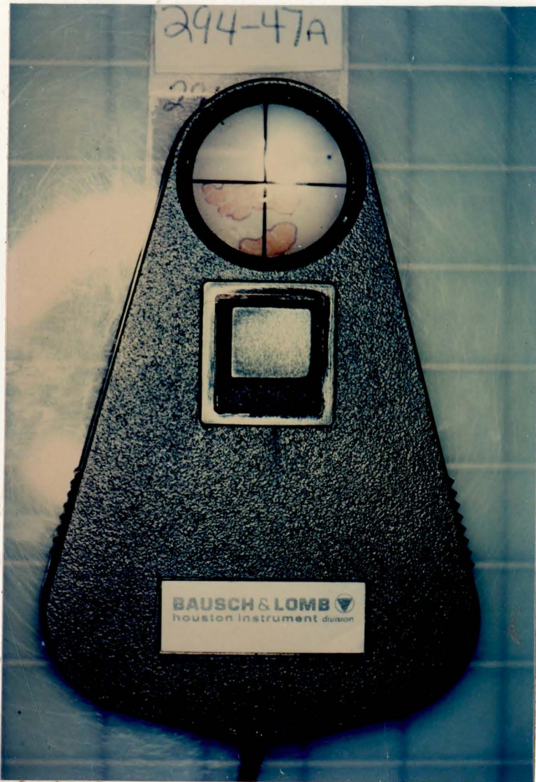
PLATE 34 - DIGITIZER HANDPIECE AGAINST THE HIPAD DIGITIZER BOARD WITH SLIDE OF TISSUE SECTION SECURED TO DIGITIZER BOARD.
