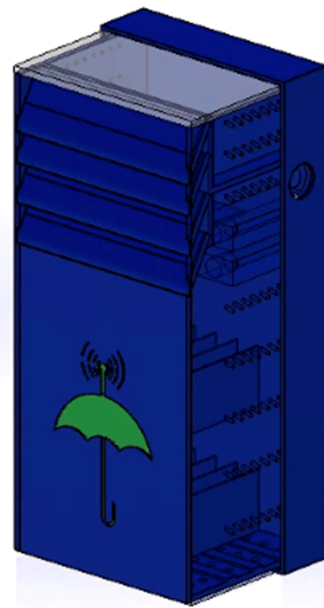
Figure 4. Umbrella Sensor Package Enclosure 3D Model - Isometric view with Transparent Side Wall for Visibility
