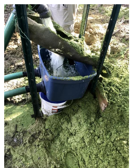
Figure 4: Current filtering system involving a hose, mesh, and catch container
