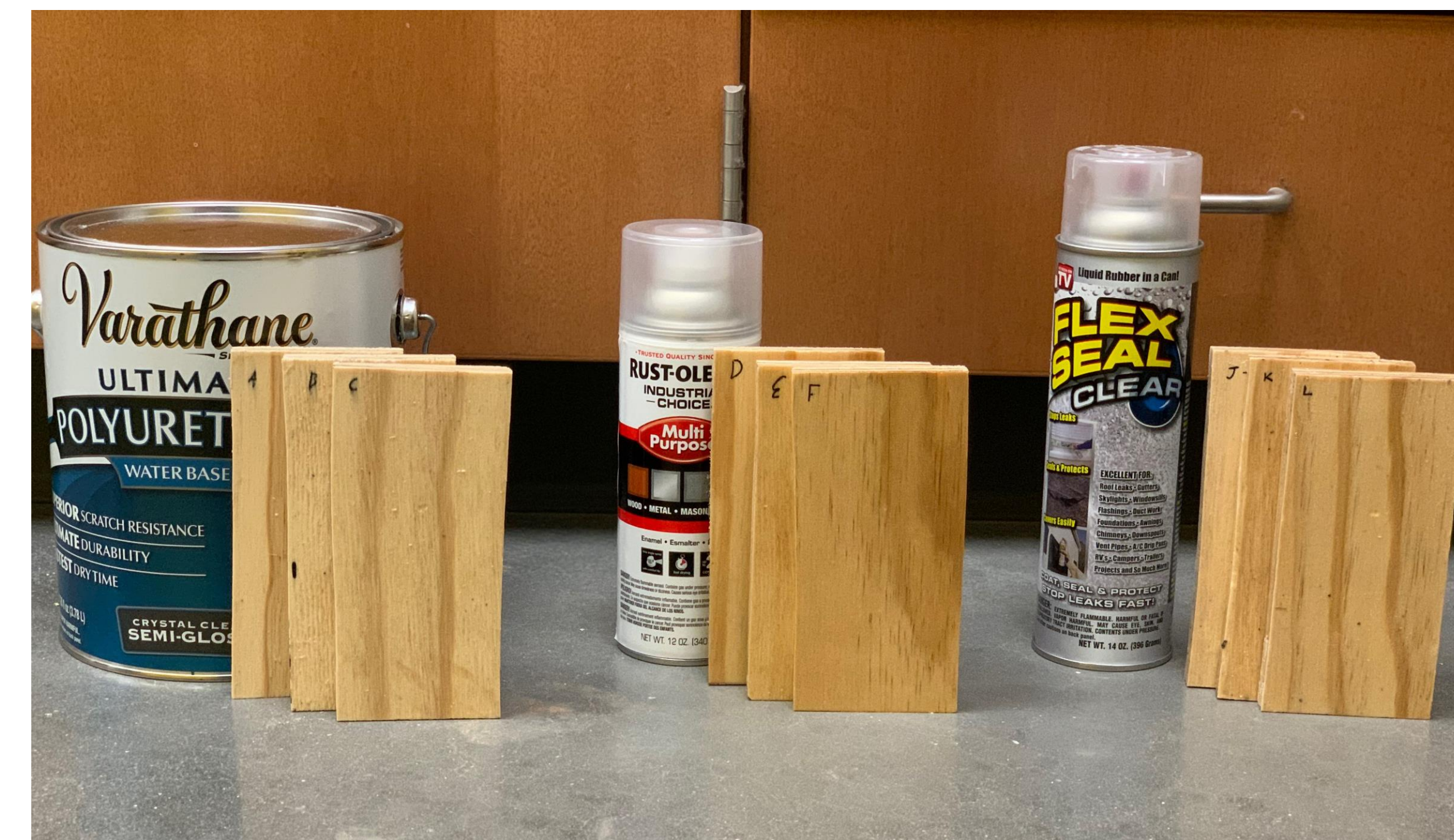
Figure 3. Final Coatings of polymers on Wood Tickets.
