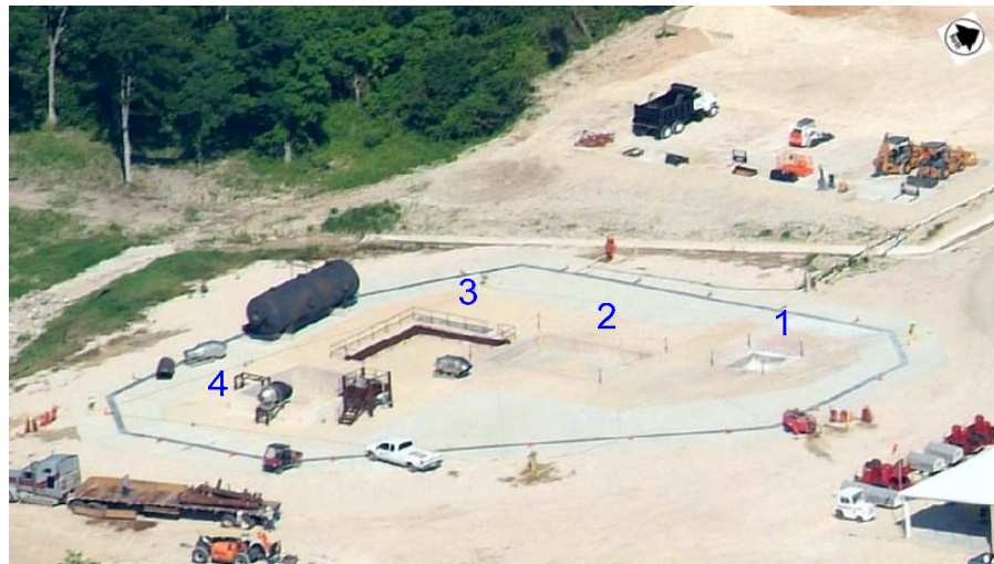
1. Small pit : 3.05 m x 3.05 m x 1.22 m 2. Large pit (65 m 2 pit) : 10.06 m x 6.71 m x 1.22 m 3. L-Trench 4. Small pit : 6.71 m x 6.71 m x 2.44 m
