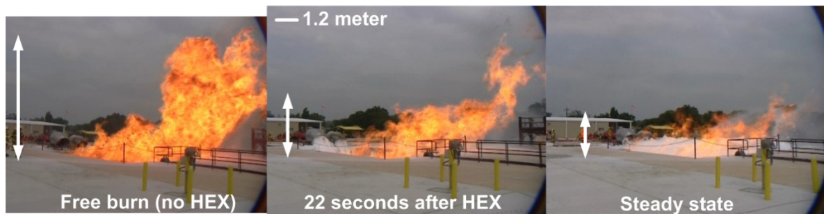
Figure 48. Fire at 65m 2 pit
