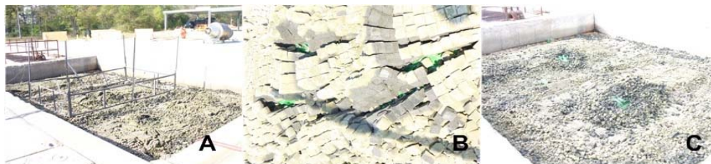
Figure 77. Foamglas condition after the experiment
