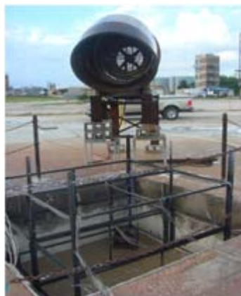
Figure 29. Test 5 - thermocouples and foam generator setup
