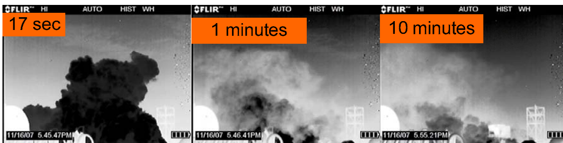
Figure 87. Methane cloud characteristics - no suppression and with expansion foam
