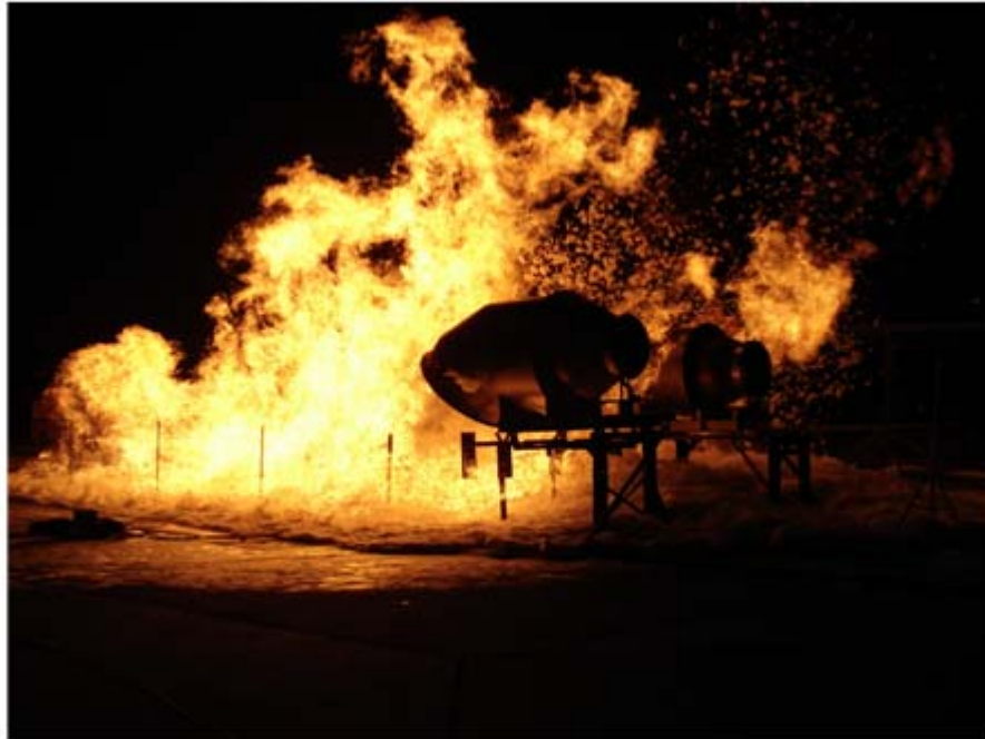
Figure 61. LNG pool fire with foam – test 6
