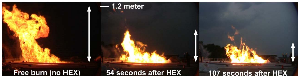
Figure 45. Pool fire on the 65 m 2 pit before and after foam application rate of 7 L/min/m 2
