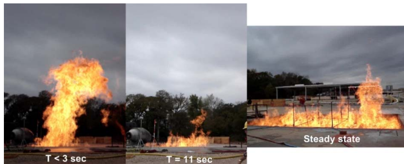
Figure 76. LNG pool fire during Foamglas® PFS application
