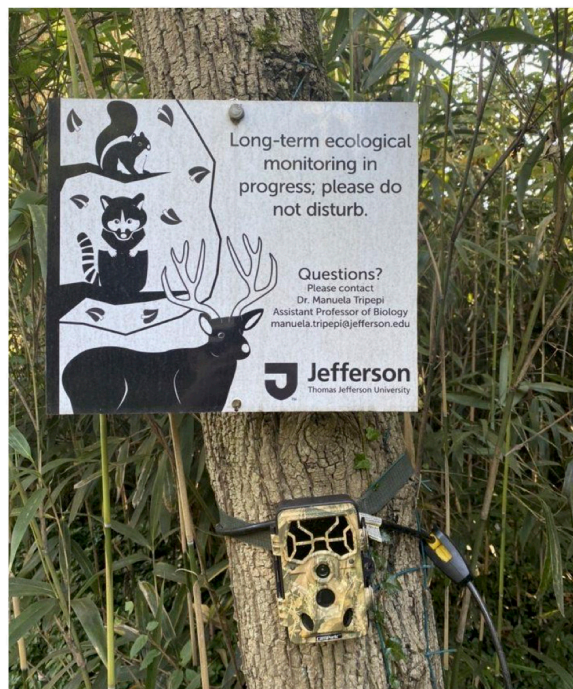
FIGURE 1. Camera set-up. The camera is secured to a tree by a strap and a master lock. A metal sign alerts passersby of the research being conducted at the site and provides contact information for the principal investigator.
