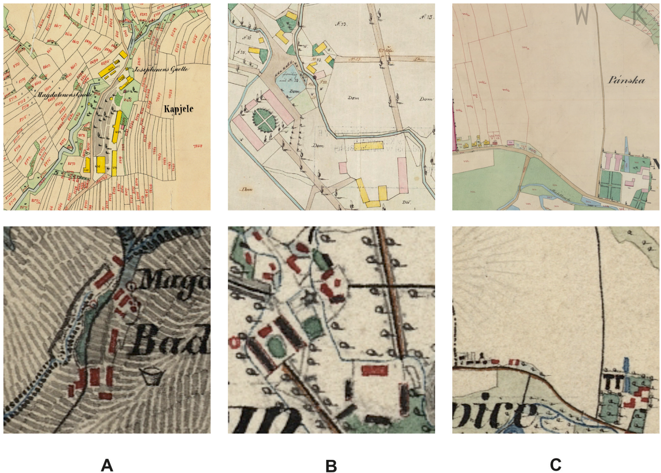
Figure 2. Comparison of cadastral 1 : 2880 maps (upper row) and Second Military Survey 1 : 28 800 maps (lower row) for Szczawnica (a), Kaniów (b), and Niewiarów (c) in Galicia (source: National Archive in Kraków, National Archive in Katowice, Austrian State Archives).
