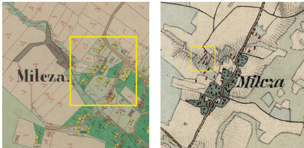
Figure 8. Comparison of a cadastral map (1851) and Second Military Survey map (1861/1862) that indicates a very high level of map generalization (source: National Archive in Przemyśl, Austrian State Archives).
