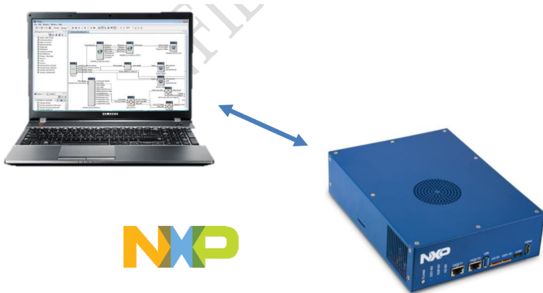
Figure 3.6. RTMaps Remote Studio connected to BLBX2
