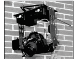
Figure 5. Unmanned aerial zeppelin with digital camera and aerial platform to control camera rotations
