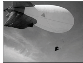
Figure 5. Unmanned aerial zeppelin with digital camera and aerial platform to control camera rotations
