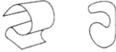
Fig. 9.1: These objects cannot be represented with an explicit form z = f(x, y)
