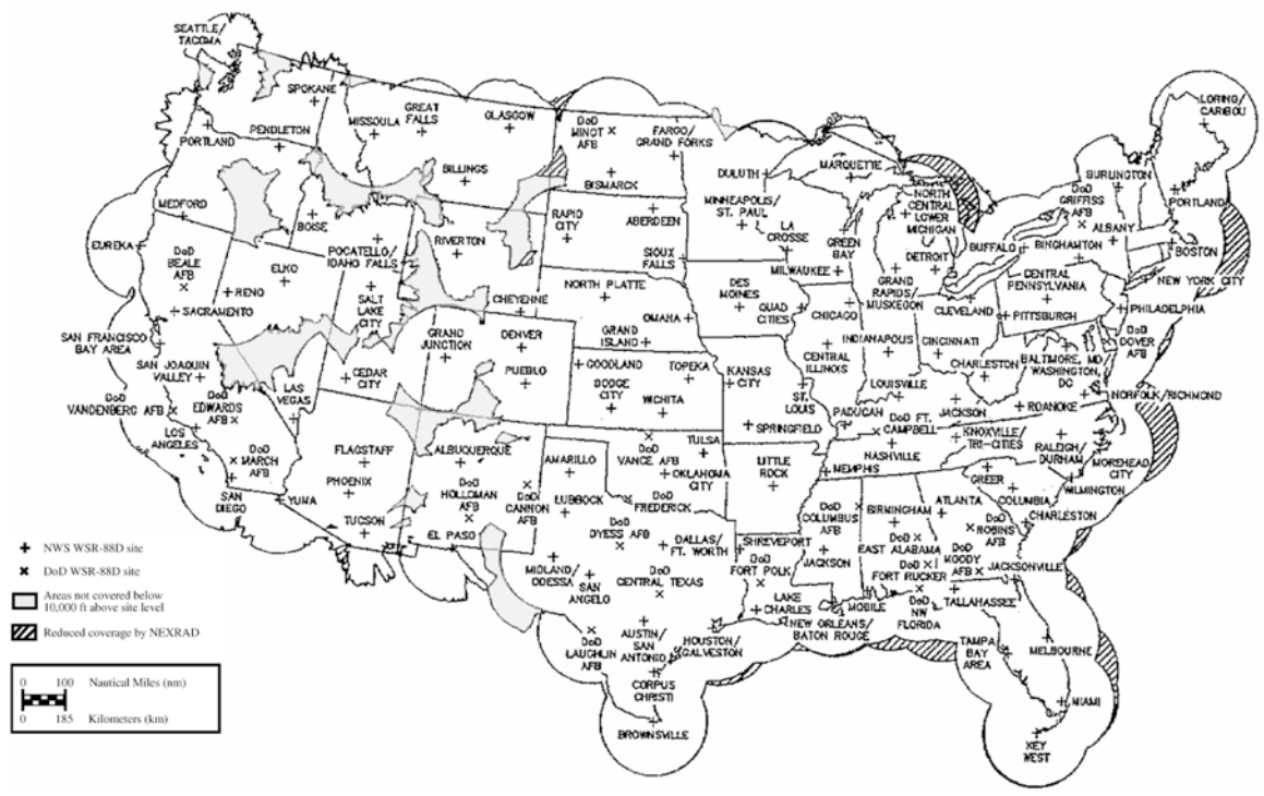
Figure 2.1. Map of WSR-88D sites within the NEXRAD network (from Serafin and Wilson 2000).
