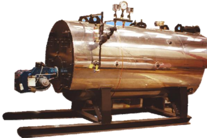
Figure 5-16: Boiler for steam generation in the pilot plant of the chemical engineering department UNAL.
