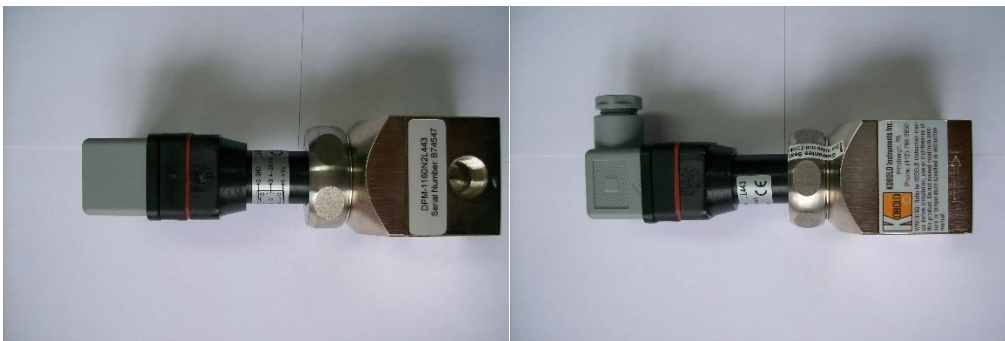
Figure 5-12: Feed flow transmitter.
