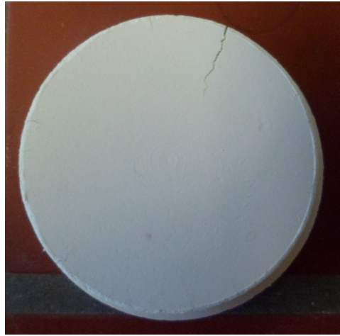
Figure 5.4: \text{Gd}_3\text{Ga}_5\text{O}_{12}:\text{Cr}^{3+} target (diameter 49 mm).
