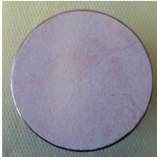
Figure 5.2: \text{CaTiO}_3:\text{Pr}^{3+} target (diameter 45 mm).
