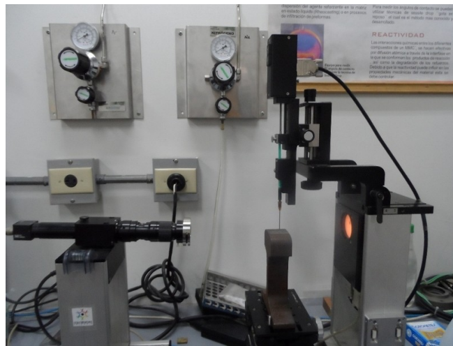
Figure 7.7: Dataphysics OCA 15. The rail sample is visible in the middle.
