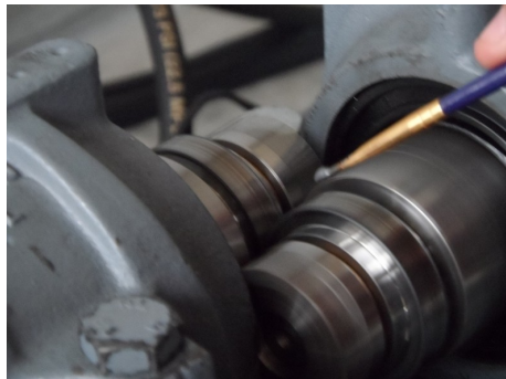
Figure 7.12: Brush method used to apply a proper film of lubricant to the sample's surface.
