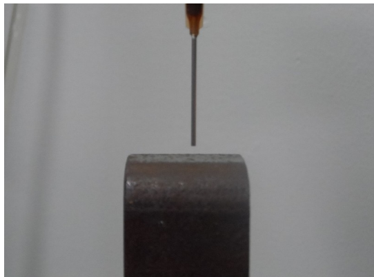
Figure 7.8: Syringe prepared for dispensing lubricant over the rail sample.
