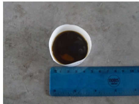
Figure 7.14: Photodegraded sample of Tribolub-1.
