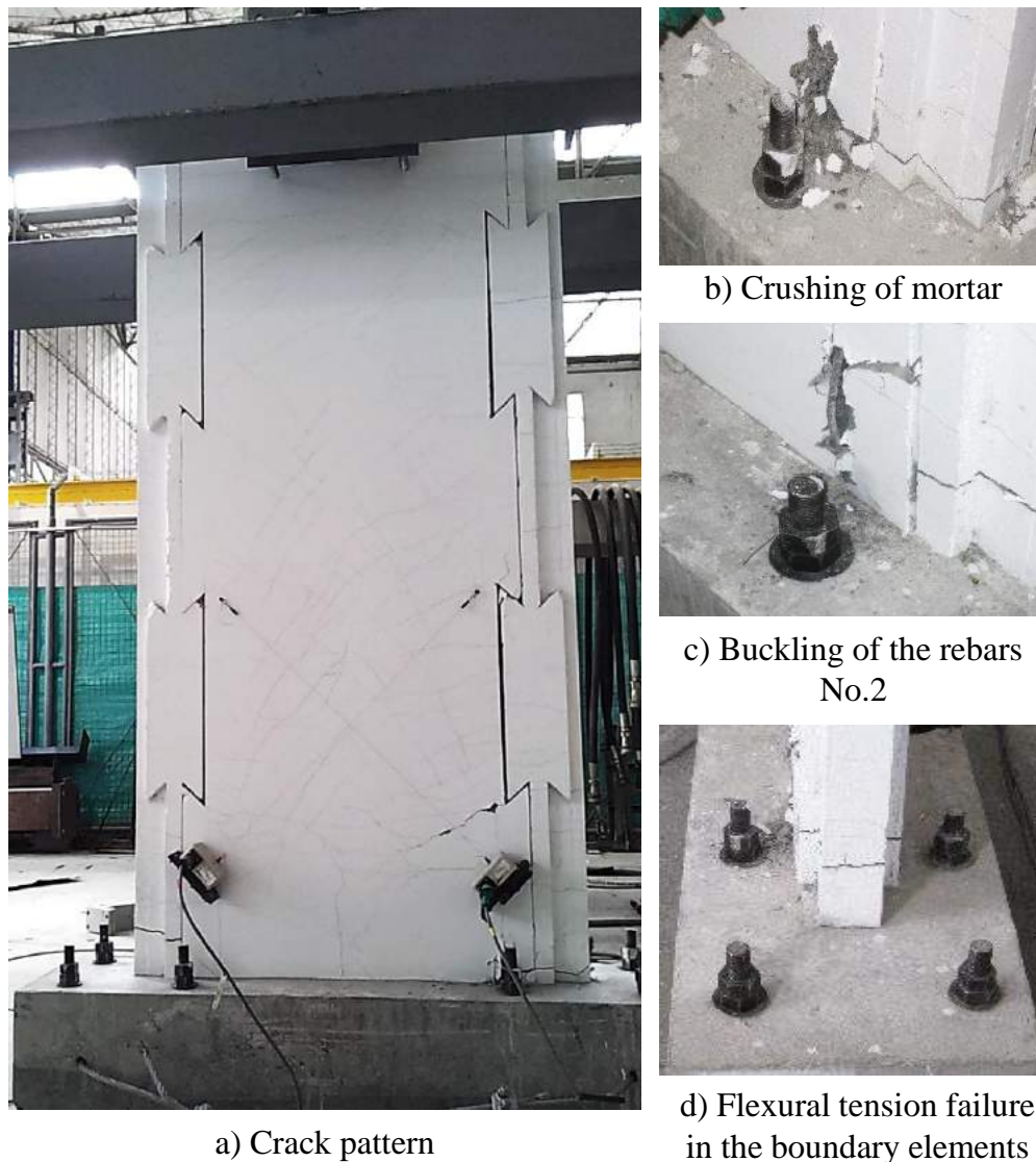
Figure 4-20: Graphical representation of the damage limit state DS 3 for the PFW
