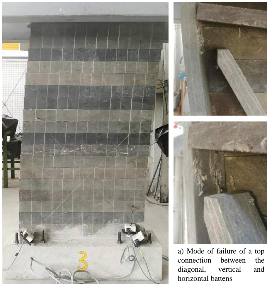
Figure 4-17: Graphical representation of the damage limit state DS 3 for the RPLW
