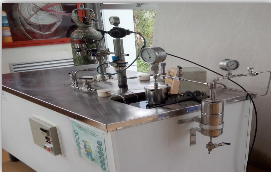
Figure 4.1. Supercritical Reactor (a)Scheme (b) Equipment
