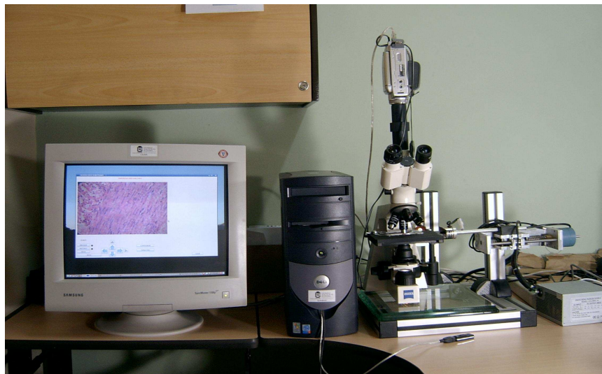
Figure 2.2: A Whole-Slide-Imaging is basically composed of a conventional optical system to which a motorized device is somehow adapted for automatic control of the stage. Likewise, a digital imaging system allows capturing the observed microscopical FOV.
