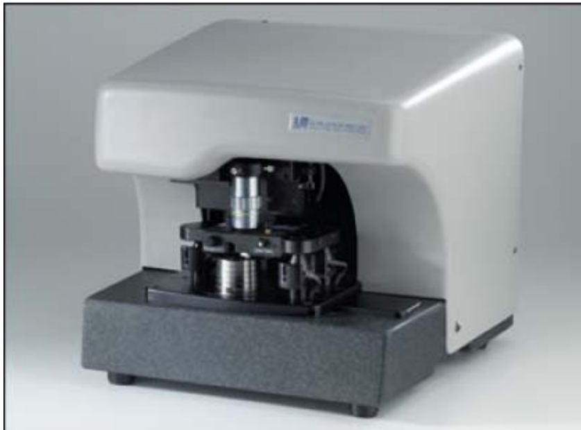
Figure 3.6: A commercial AFM (Pacific Nanotechnology Incorporated) from Dr. Liang's surface science and interface laboratory. [69]
