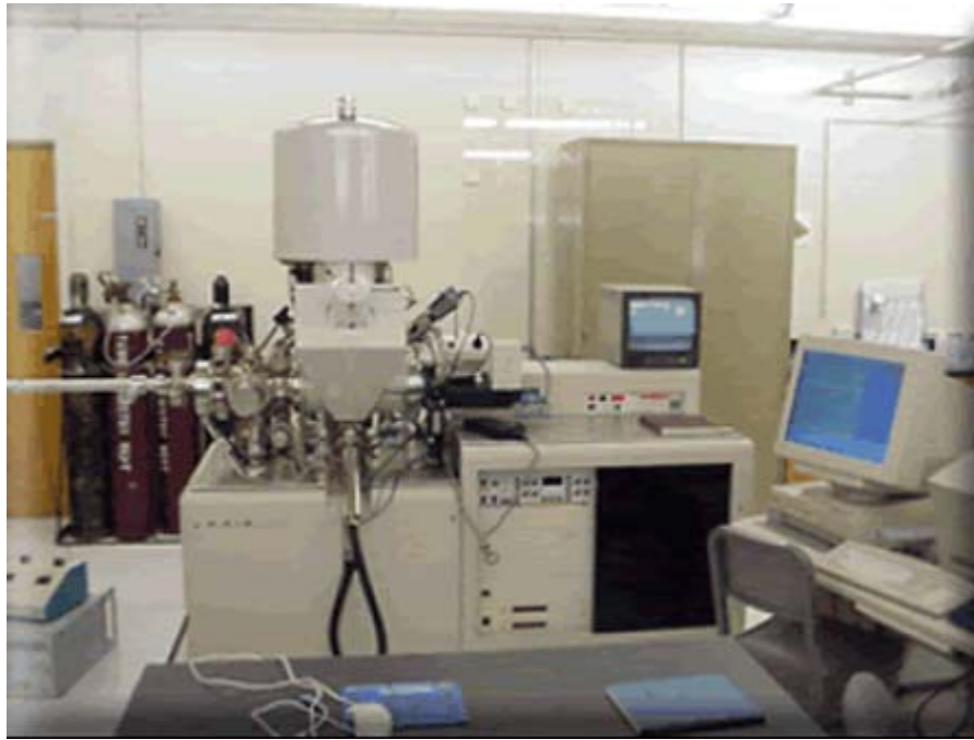
Figure 3.9: A Kratos Imaging X-ray Photoelectron Spectrometer in Materials Characterization Facility. [69]
